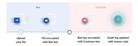
Customer keys are hosted by our partner, AWS, in systems that are designed with 99.9999999% durability and deployed in multiple availability zones. Decrypted data and encryption keys (both the Customer key and the Box key) are only stored in memory and never stored on disk.
