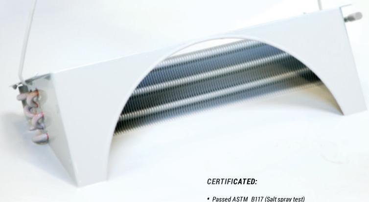
Process that guarantees 100 % penetration & protection. The entire coil is immersed into a liquid form of LCE Coating letting the liquid penetrate even the smallest spaces between fins including fin collar, louvre, heat slots or any other type of forming. In addition, all other parts like U-bends, end-plates, side plates, headers, capillaries are coated and protected as well.
