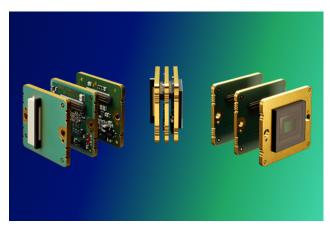
The new VC Power SoC is an FPGA accelerator for onboard image pre-processing, that is firmly integrated into the design of the VC MIPI Camera Modules. It is available as an option for all VC MIPI Cameras.
