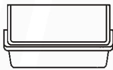
Bucket with front lip reinforcement
