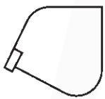
Bucket with front lip reinforcement
