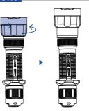
**@USB-C Charging Port** Rotate the neck to open the charging port.
