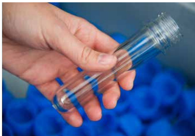
Preforms for mobile water bottling WBP 1300
