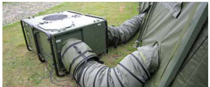
MAC 18 – Air conditioning unit
