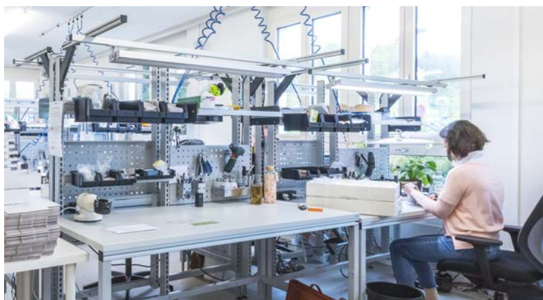
Height-adjustable assembly workstation and transport trolley with electric motor
