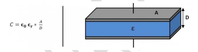
Capacitance is proportional to the area of overlap but inversely proportional to the separation between the conducting sheets. The bigger the area of overlap is and the closer the sheets are to each other, the greater is the capacitance.
