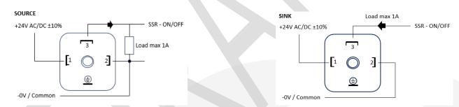
When liquid is present the switch toggles the SSR contact, the SSR contact can be configured as NO (Normally open) or NC (Normally closed). The initial state is when there are no liquid surrounding the switch.
