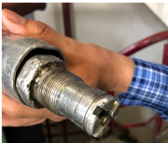
Damage to threads on SDX 3 Nozzle
