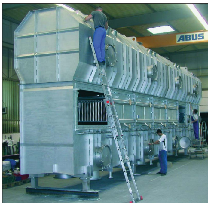
Figure 28: Fluid-bed dryer, fluid-bed area 26 m 2 , with integrated slide-in steam coils for a detergent intermediate product
