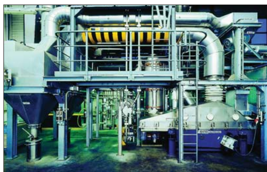
Figure 24: Natural frequency fluid bed dryer/cooler 22 m² area
