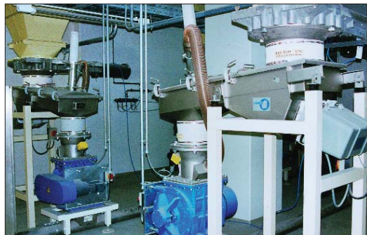
Figure 13: Bin discharging trough conveyors with electromagnetic vibrators
