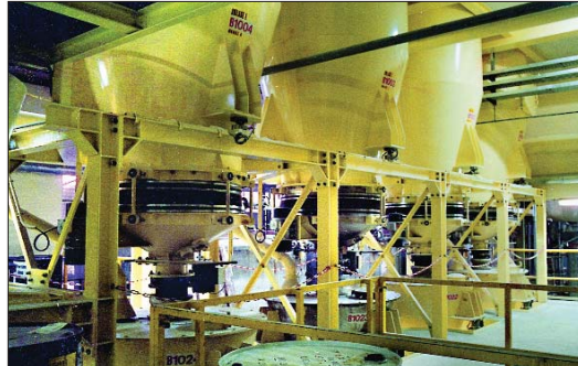
Figure 12: SX bin dischargers in a detergent factory
