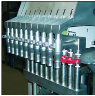
Figure 11: ER batching conveyors in special design for proportioning of catalyst granules
