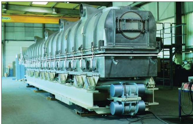
Figure 24: Natural frequency fluid bed dryer/cooler 22 m² area
