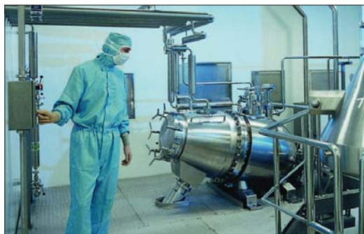
Figure 8: Screening machine suitable for CIP and sterilization (Works photo Schering AG)
