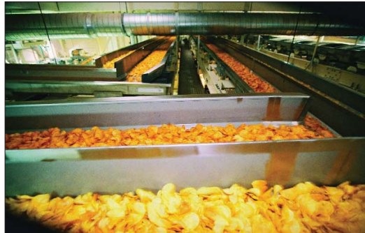
Figure 3: Partial view of a vibrating conveyor plant with an overall length of 120 m used to convey potato chips at a rate of 60 m³/W.
