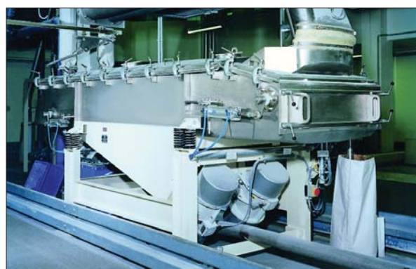
Figure 9: SR 36/10 screening machine in a food processing factory
