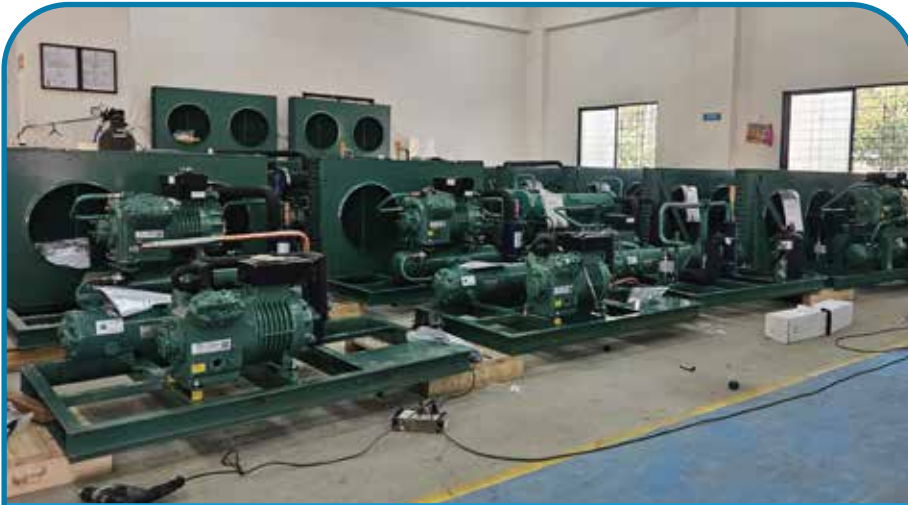
Condensing Unit (Bitzer)
