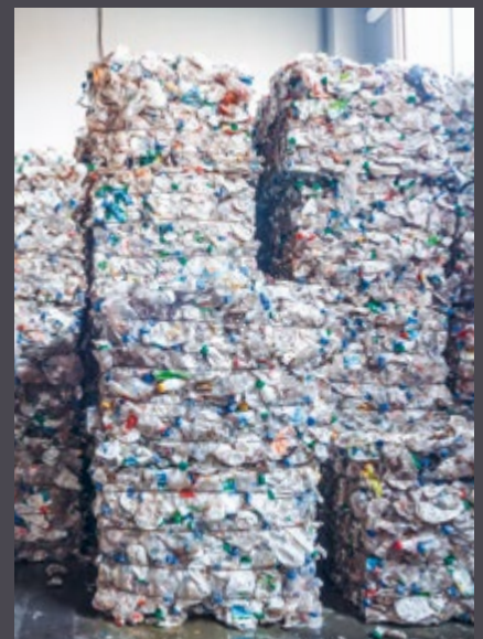
The sorted packaging arrives in bales. To produce hanit, our method also uses mixed plastics that are not recycled by conventional recycling methods.
