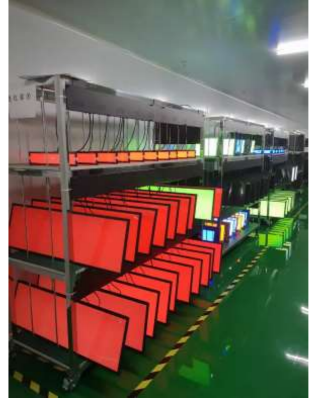
Aging Test Room
