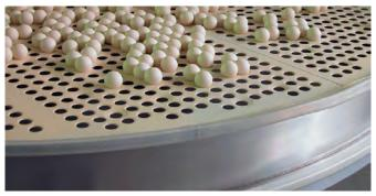
Ball tray for screen cleaning balls, made of stainless steel or carbon steel
