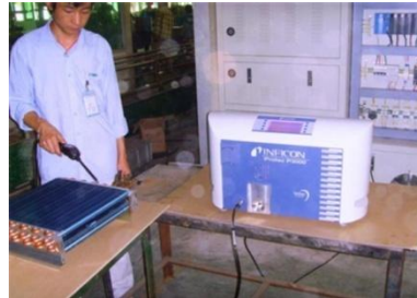
Precise helium inspection for leakage
