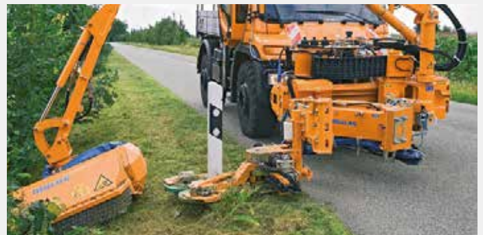
Reflector post mower mounted on a combination mower
