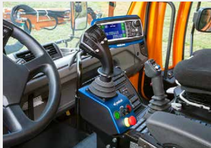
m|pilot multifunction joystick with 6-fold proportional control
