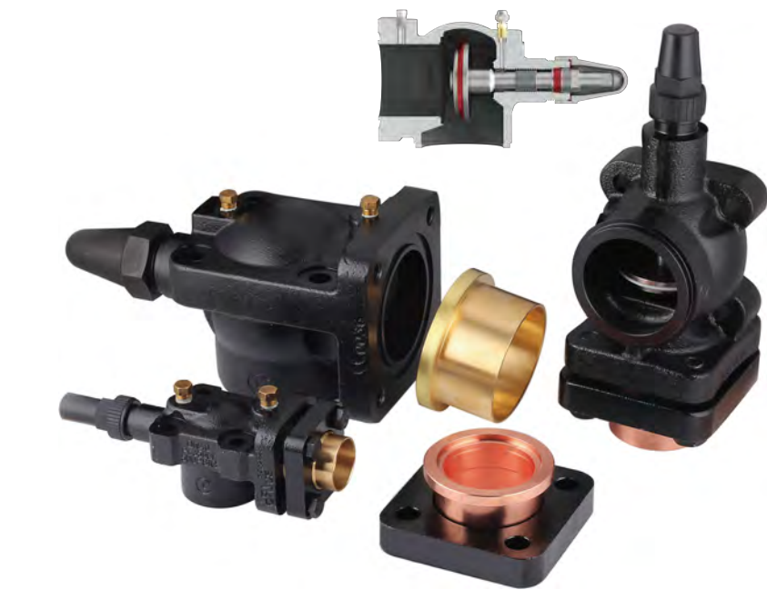
铸铁吸排气阀 Cast iron suction and discharge valve 制冷剂 Refrigerants: CFC, HCFC, HFC 温度范围 Working temperature range: -40°C ~ +140°C 规格尺寸 Specification and size: DN25 ~ DN125 压力范围 Pressure range: 0 ~ 4.0 MPa ( 液压hydraulic pressure 6.0 ) 优特点 Features and advantages: 耐低温球铁材质 low temperature resistant ductile iron 压降低 low pressure drop 双密封 dual seal 耐用寿命 long service life UL and CE certifications
