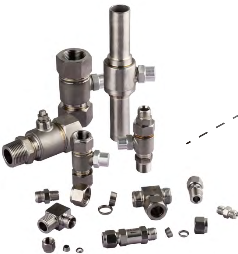
高压球阀 High pressure ball valve 制冷剂 Refrigerants : CFC, HCFC, HFC, R744 温度范围 Working temperature range : -40℃ ~ +140℃ 规格尺寸 Specification and size : DN4 ~ DN40 压力范围 Pressure range : 0 ~ 16.0 MPa 优点 Features and advantages : 全不锈钢材质制造 full stainless steel 特氟龙迷宫式密封 labyrinth packing of PTFE 流道呈直通型无压降 The flow channel is straight without pressure drop CE CERTIFICATION
