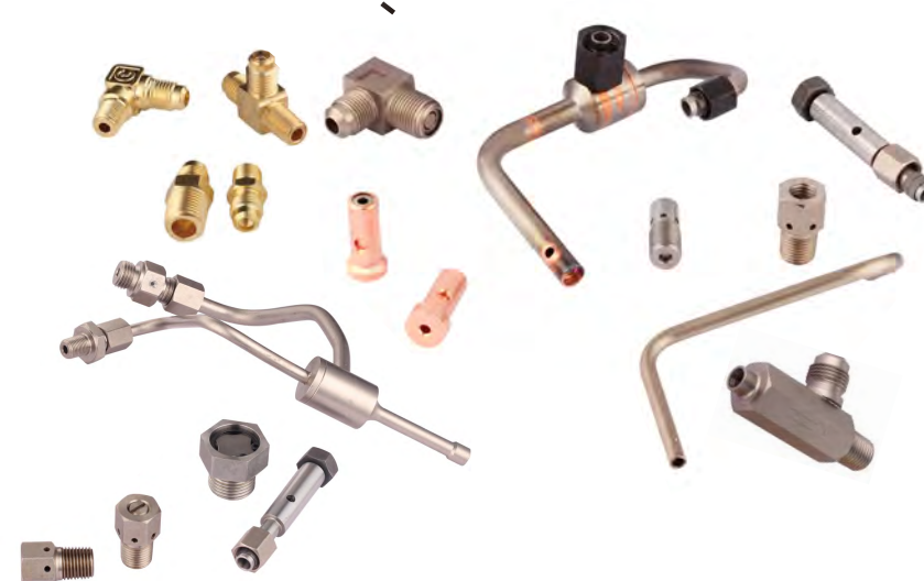
功能接头 Functional connector 制冷剂 Refrigerants: CFC, HCFC, HFC 温度范围 Working temperature range: -29°C ~ +120°C 规格尺寸 Specification and size: DN1 ~ DN25 压力范围 Pressure range: 0 ~ 4.5 MPa ( 液压hydraulic pressure 6.3 ) 优特点 Features and advantages: 特氟龙预涂密封良好 Pre-glued PTFE has a good sealing performance 无氧钎焊坚固耐用 Oxygen-free brazing will make products sturdy and durable 精度高 high precision 可靠性强 strong reliability CE certification
