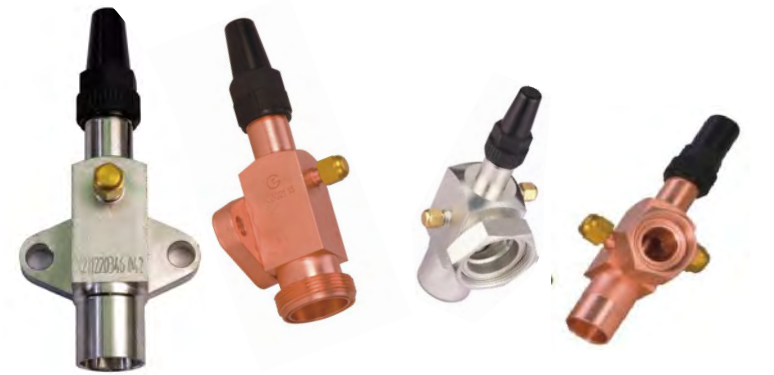
吸排气阀 Suction and discharge valve 制冷剂 Refrigerants: CFC, HCFC, HFC 温度范围 Working temperature range: -40°C ~ +140°C 规格尺寸 Specification and size: DN4 ~ DN50 压力范围 Pressure range: 0 ~ 4.5 MPa ( 液压hydraulic pressure 6.3 ) 优特点 Features and advantages: 耐低温材料 low temperature resistant material 耐用寿命 long service life 压降低 low pressure drop 双密封 dual seal UL and CE certifications
