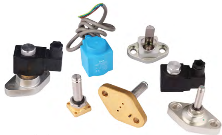
法兰电磁阀 Flange solenoid valve 制冷剂 Refrigerants: CFC, HCFC, HFC 温度范围 Working temperature range: -40°C ~ +100°C 规格尺寸 Specification and size: DN1 ~ DN10 压力范围 Pressure range: 0 ~ 3.0 MPa 优特点 Features and advantages: 无焊锡整体加工 Welding free and overall processing 抗震耐操无外漏 shock-and damage-resistant, no outside leakage 寿命长 long service life ( 1500万次无泄漏 no leakage after 15,000,000 cycles ) CE certification
