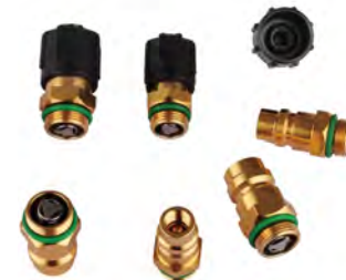
介质冲抽阀 Medium charging and evacuating valve 制冷剂 Refrigerants : CFC, HCFC, HFC 温度范围 Working temperature range : -40℃ ~ +120℃ 规格尺寸 Specification and size : DN2 ~ DN6 压力范围 Pressure range : 0 ~ 4.5 MPa 优点 Features and advantages : 双重密封无泄漏 dual sealing without leakage 操作方便 easy operation 重复使用寿命长 long service life CE CERTIFICATION
