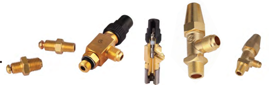
介质充抽阀 Medium charging and evacuating valve 制冷剂 Refrigerants: CFC, HCFC, HFC 温度范围 Working temperature range: -40°C ~ +120°C 规格尺寸 Specification and size: DN3 ~ DN15 压力范围 Pressure range: 0 ~ 4.5 MPa ( 液压hydraulic pressure 6.3 ) 优特点 Features and advantages: 特氟龙预涂密封良好 Pre-glued PTFE has a good sealing performance 方向接头使用方便 Universal joint is easy to use 耐用寿命 long service life 双重密封无泄漏 dual seal and no leakage CE certification
