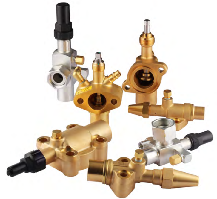
吸排气阀 Suction and discharge valve 制冷剂 Refrigerants : CFC, HCFC, HFC 温度范围 Working temperature range : -40℃ ~ +140℃ 规格尺寸 Specification and size : DN4 ~ DN50 压力范围 Pressure range : 0 ~ 4.5 MPa ( 液压 hydraulic pressure 6.3 ) 优点 Features and advantages : 耐低温材料 low temperature resistant material 耐用寿命长 long service life 压降低 low pressure drop 双密封 dual seal UL and CE certifications
