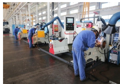
Pipe automatic welding
