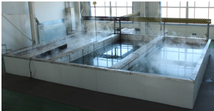
Specially designed degreasing tank
