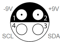
Probe’s power supply pin assignment “cable view”
