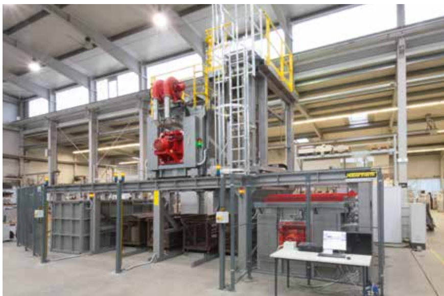
Mobile drop-bottom furnace for solution annealing with pit-type furnace for artificial ageing with four parking places
