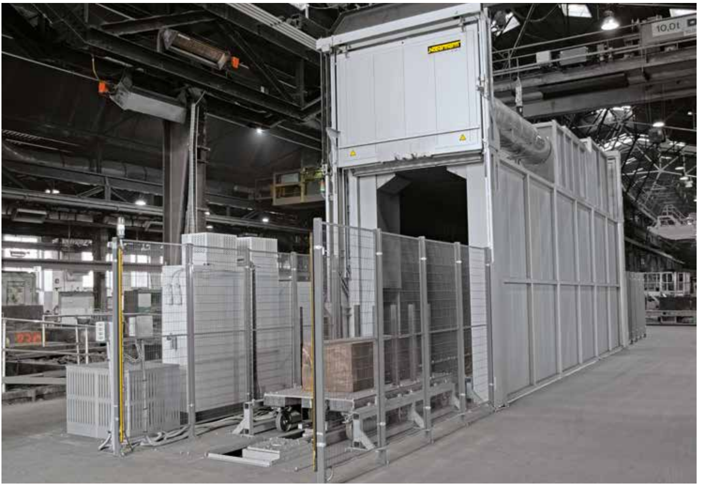
Continuous pilgrim step furnace system NBI 70000/15HAS for black wash drying on sand cores
