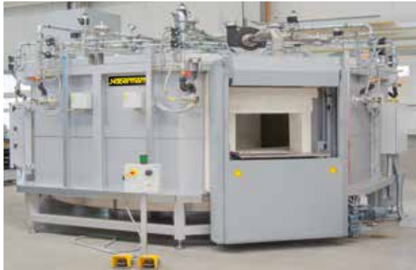
Gas-fired rotary-hearth furnaces for preheating of ceramic moulds up to 1100 °C incl. thermal post combustion for exhaust gas cleaning
