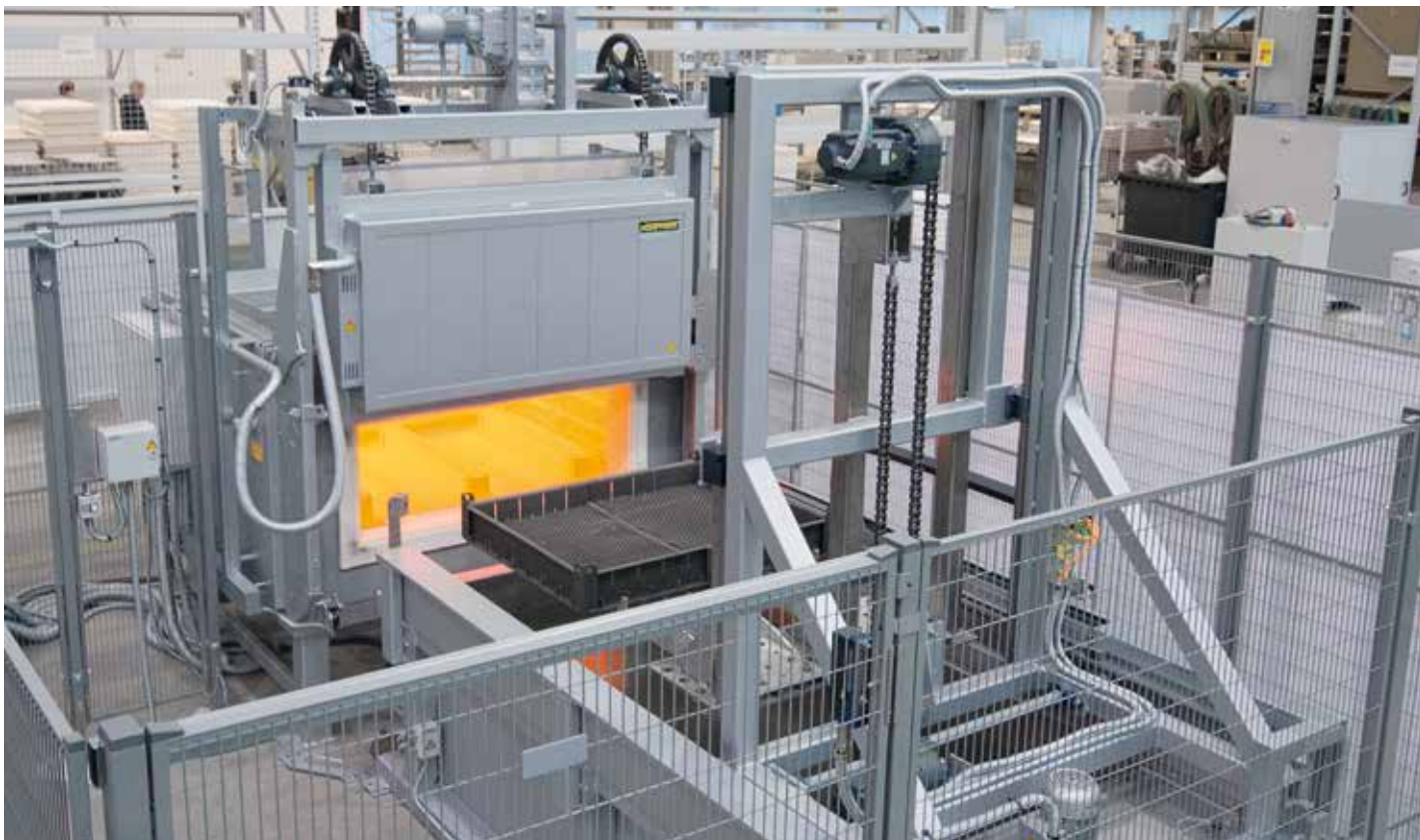
Automatic quenching and tempering plant N 644/S
