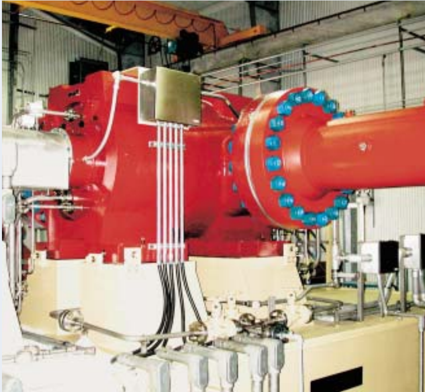
Fig.7 Natural gas compressor.
