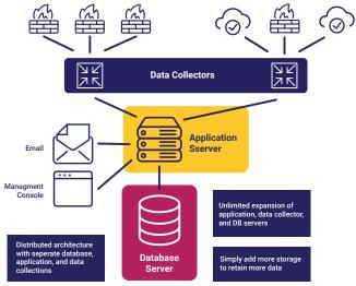
A distributed architecture allows easy expansion of any FireMon element enabling the platform to scale to the needs of any organization.
