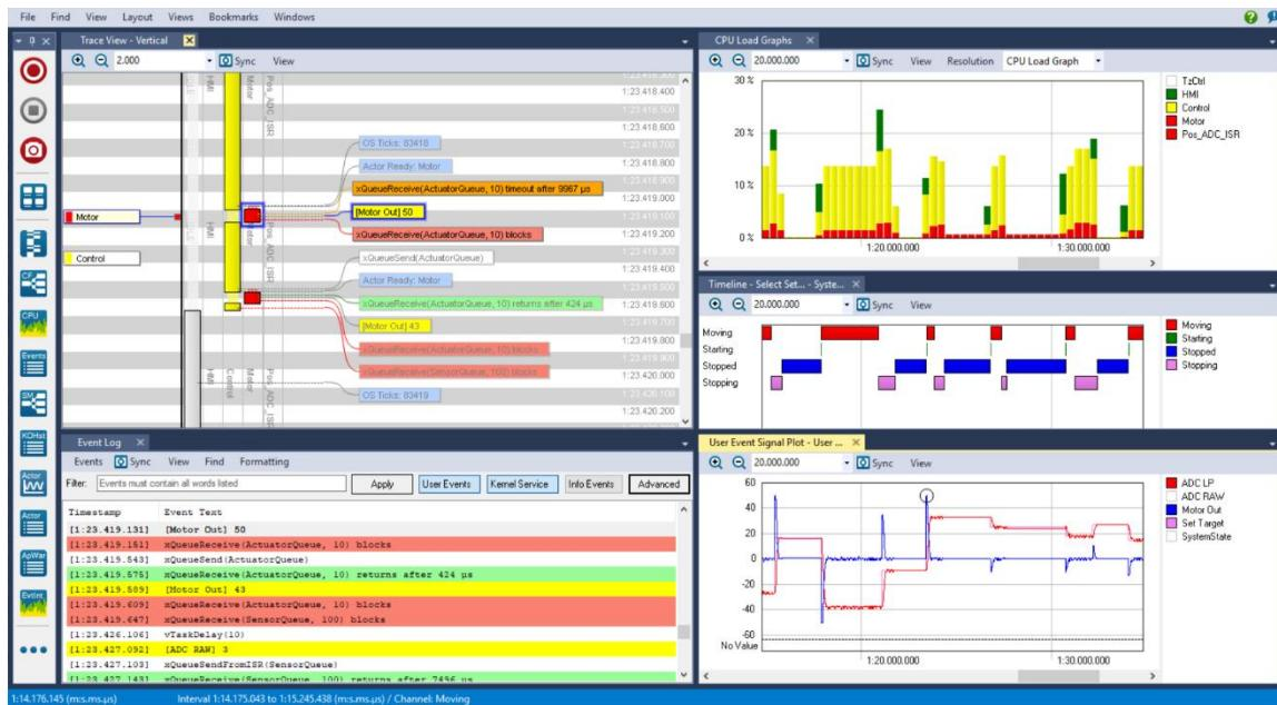
*Caption: Tracealyzer provides multiple synchronized views of runtime behavior – helping engineers connect the dots between CPU load, task timing, and system events.*
