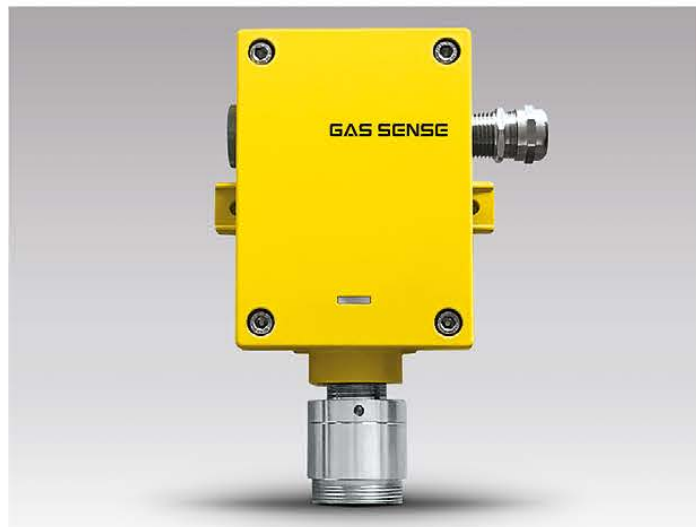
GDPC – ATEX certified gas detector for combustible gases ATEX marking: \text{Ex} II 2G Ex db IIC T4 Gb \text{Ex} II 1G Ex da IIC T4 Ga
