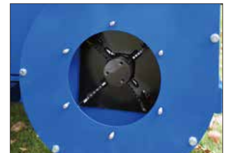
All steel impeller reduces the volume of leaves to a fraction of their original bulk
