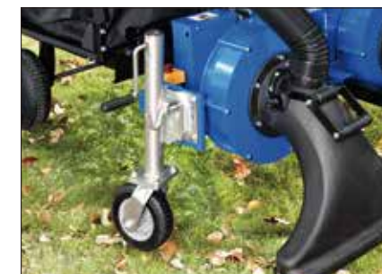
Foldable trailer jack can adjusting the height of the leaf vacuum snouts
