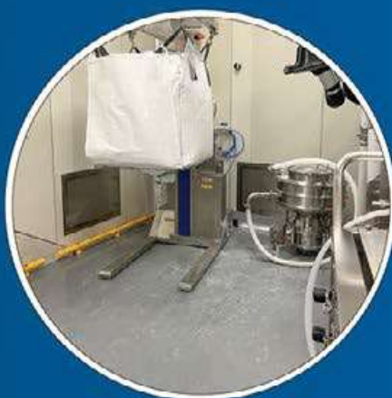
Mobile Lifting Column for Big Bag Unloading
