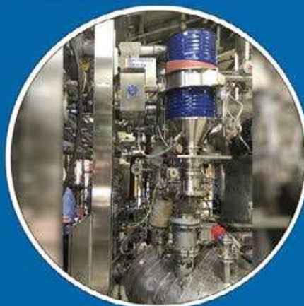
Fixed Automatic Drum Lifter for Reactor Loading
