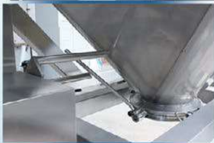
Automatic Valve Opening System
