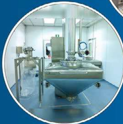
Bin Blending Column for Mill loading
