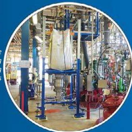
Big Bag Discharge Station for feeding reactor using Vacuum Conveyors
