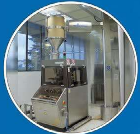
Stationary Automatic Drum Lifter for Packaging Machine Loading
