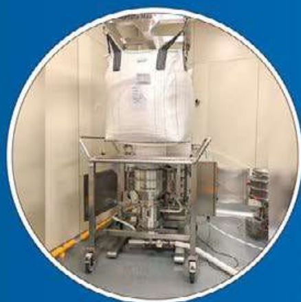
Mobile Closing System integrated with CIP
