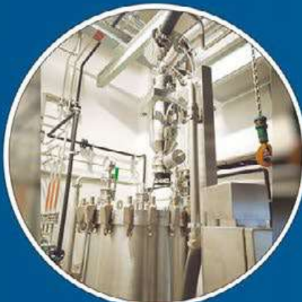
Lifting Column with Vacuum Conveyor for Plate Filter Loading
