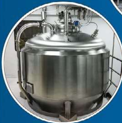
Jacket Hoppervac in sterile area
