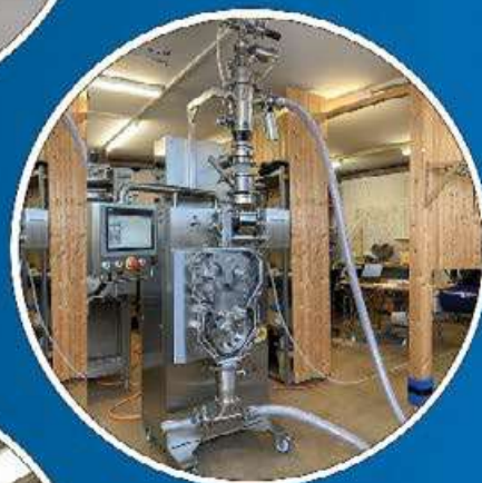
Vacuum Conveyor to load a Roller Compactor
