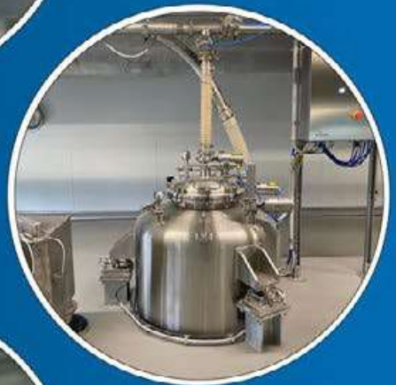
Vacuum Conveyor Hoppervac on a fixed column which discharge in drums
