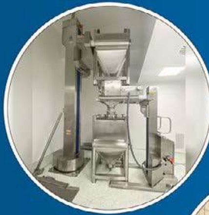
Blending and discharging System from Bin-to-Bin by Mill
