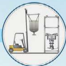
Frame with sockets for forklift connection Used to lift and position Big Bags without using the forklift
