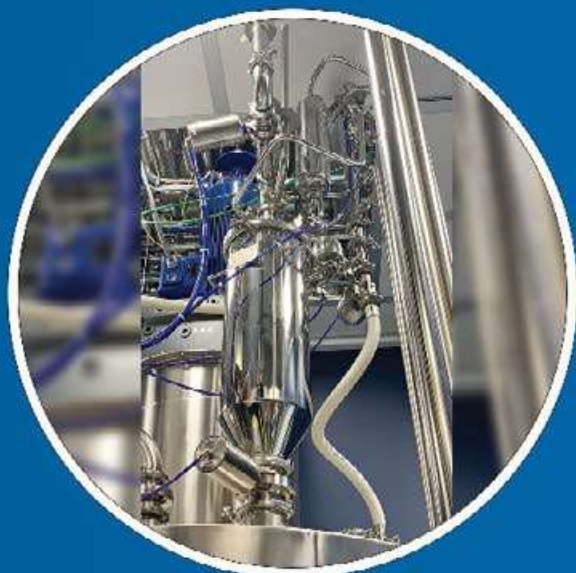
Filtervac FT200 for reactor charging
