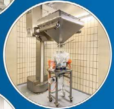
Bin Blending Column for Mill loading
