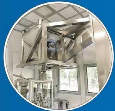
Lifting Column for Bin with an integrated vibration system
