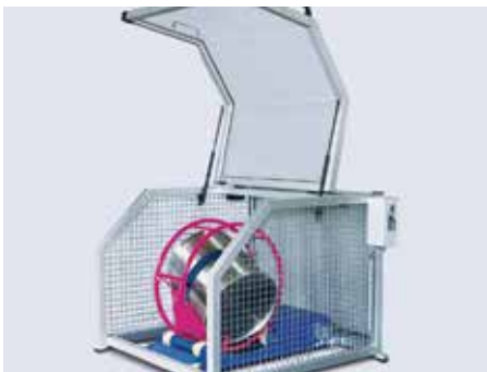
Protective hood made from aluminum mesh and perspex
