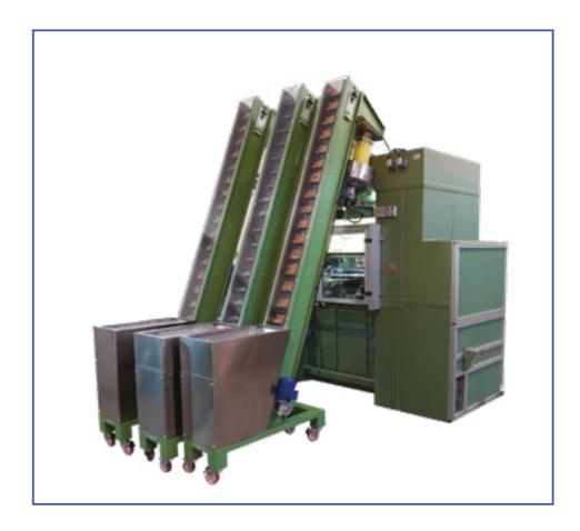
NOTE: the press CB/60/7+7/65/125 is able to produce, starting by the cup: 240/min bullets 9 mm or
