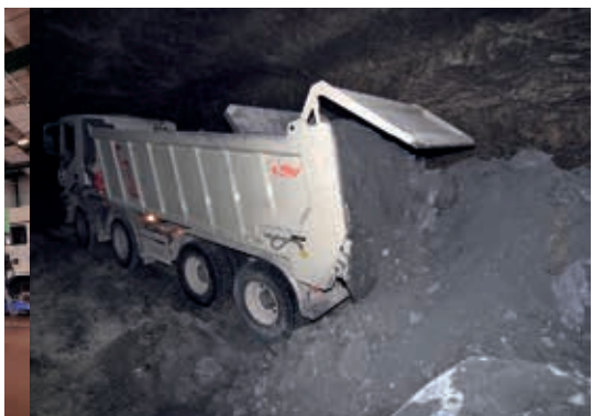
Underground use in salt mine: transport of backfill materials
