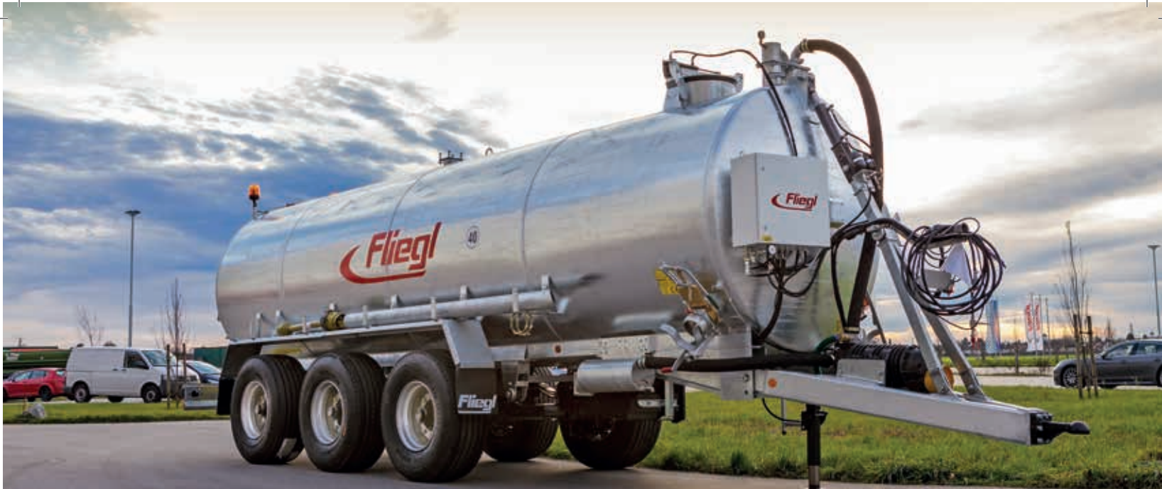
Water tanker with hose reel and sprinkler nozzle
