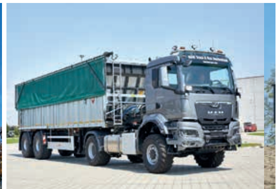
Toplift Light: sideways-folding cover net
