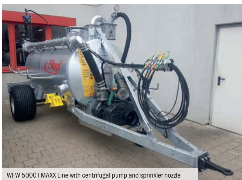
Hydraulically swivelling sprinkler nozzle
