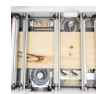
4 cutterheads Mould and plane four sides simultaneously
