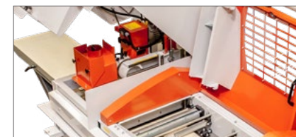
The additional fifth cutterhead for moulding With the feature of adjustable tilt angle up to 270° and a sliding feature in horizontal and vertical axis.
