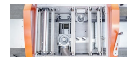
Five feed rollers Four steel rollers and one polyurethane roller move material through the machine
