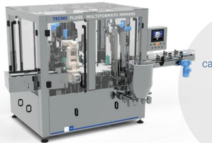
Multiformats filling and capping monoblocks with quick size changeover. Output from 1.500 to 3.000 pcs/h.
