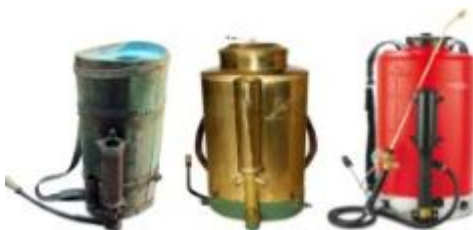
Development of backpack sprayers (from left to right): Device from 1892, 1950, 1977
