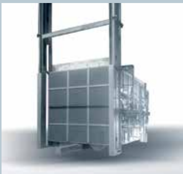
Bogie hearth furnace for the thermal post-processing of steels. Output: 2.500 kW
