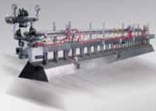
Heating system to dry rug cloth webs. Output: 1.500 kW
