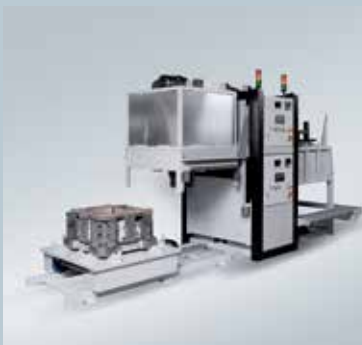
Heating system to preheat casting tools in wheel rim casting. Output: 100 kW
