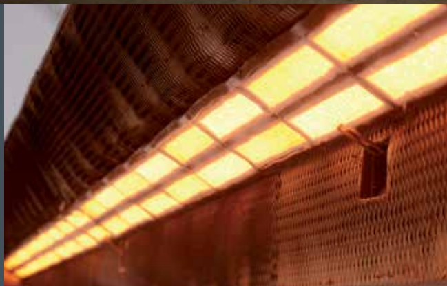
Burner, linear modular design. W x H = 5.5 m x 0.1 m, output 500 kW
