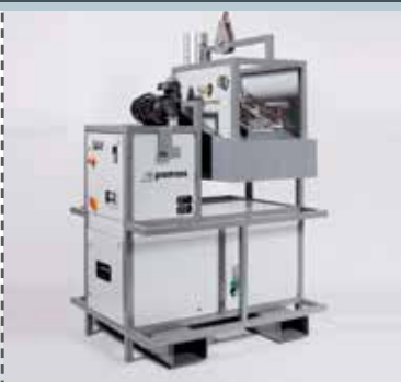
Heating system with a station to preheat pouring spouts. Output: 350 kW
