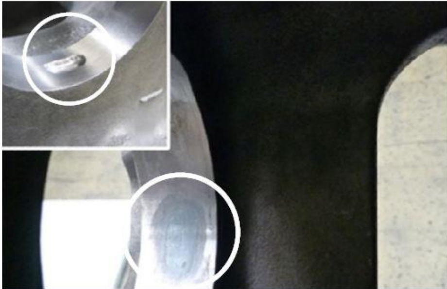
Cold spray repair after 12,600 hours
