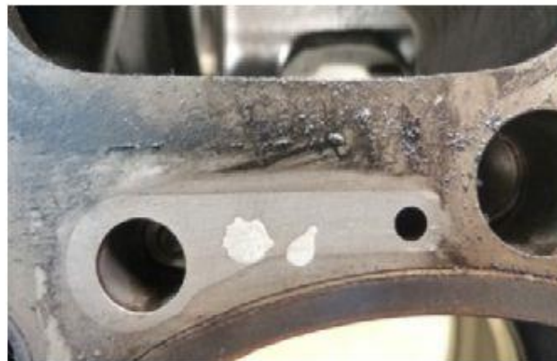
Resurfaced & repaired with D523
