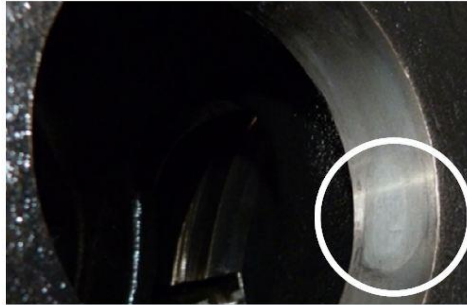
Cold spray repair after 24,600 hours
