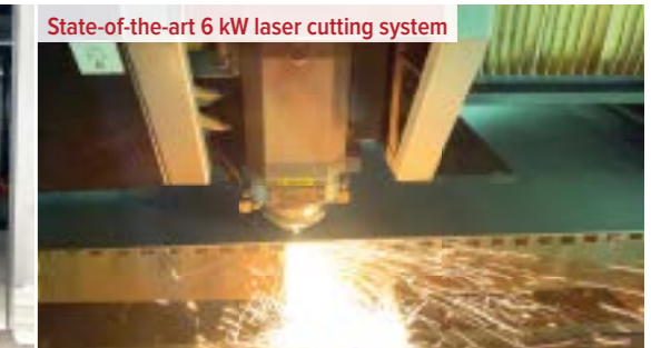
State-of-the-art 6 kW laser cutting system
