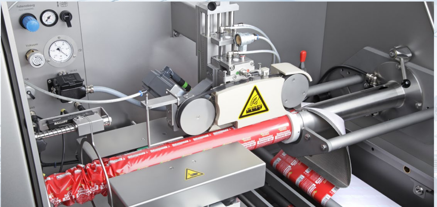
The hot-sealing station of the TSCA provides reliable sealing.
