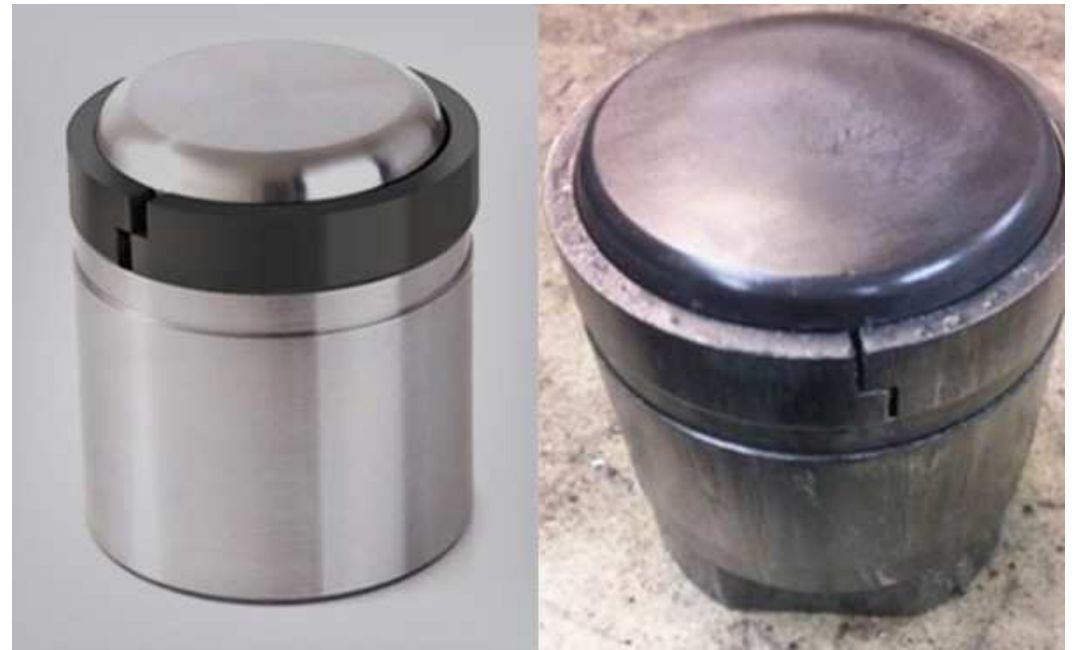
iTherm® Plunger: new (left) and after 120.000 shots and 3 ring replacements (right)
