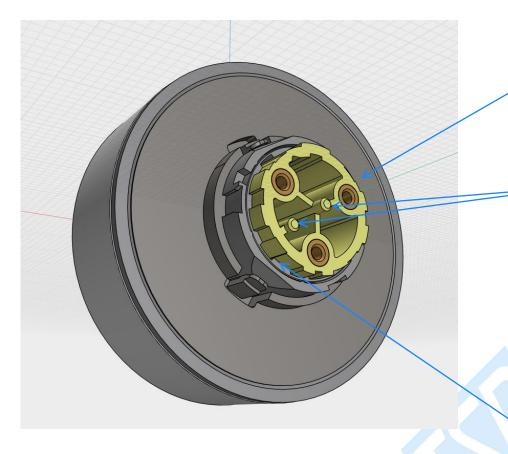
Injection-molded copper nuts: Compared to hotpressed copper nuts, inserting the copper nut during injection molding ensures it won't fall off, significantly reducing the risk of detachment due to environmental changes and rough handling.
