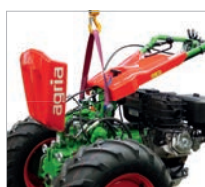
Safe loading with lifting sling and eye bolts
