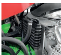
Additional oil cooler for use even at high temperatures
