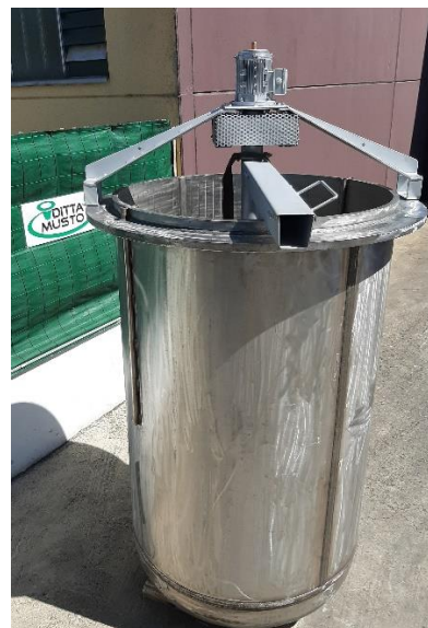
RECYCLING CRUCIBLE FOR ZINK ALLOYS, CAPACITY 13000 KGS
