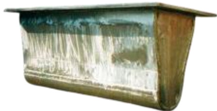
CRUCIBLE FOR ZINK RECYCLING, CAPACITY 2500 KGS
