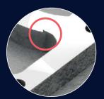
**■** Finishing Superficial finishing degree and completeness control for possible defect on the weft or lapping
