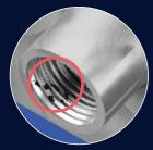
Internal porosity -Porosity control inside less than 10mm diameter holes
