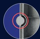
Checking the opening of holes and interception of occlusions (even partial) due to the presence of burrs or broken plugs
