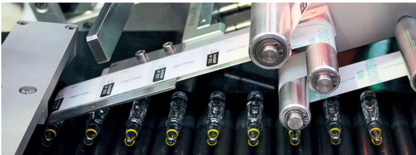
Figure 2: Ampoule Labeler (Labeler Model RML)
