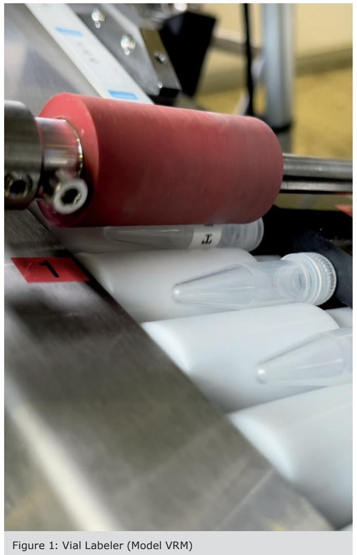
Figure 1: Vial Labeler (Model VRM)
