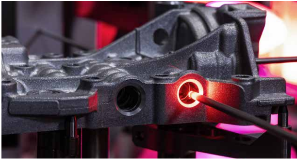
Inspection of small bore surfaces of a valve housing
