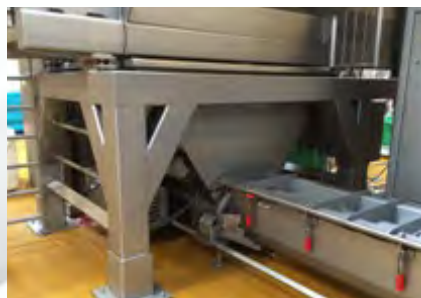
Horizontal screw shown with closed lid.
