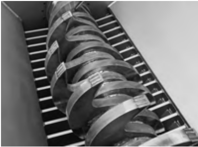
Crusher claw(s) made of mild steel with hard ended claw tips.
