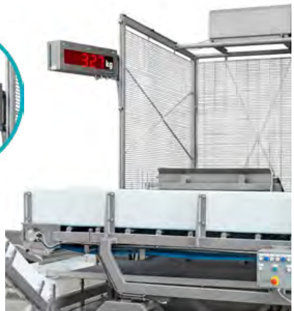
Details showing drip trays and weighing/load cells.
