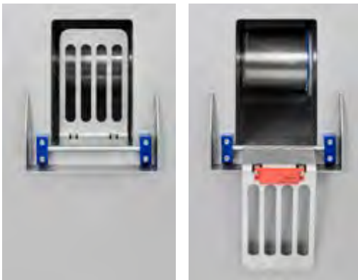
A prime example of scansteel foodtech® hygienic design is given by the hygienic zone positioned between the worm/auger and the gear box. Hygienic zone shown in running position (closed) and in cleaning/inspection position. When opened, the grinder cannot be started until the guard has been positioned in closed position.
