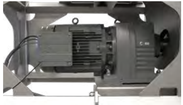
The scanStructor is typically equipped with a 37 kw motor.
