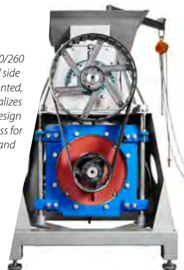
SuperGrind 400/260 shown with all side panels dismantled, side view. Designed for easy access at maintenance and inspection. The automatic greasing system for main bearing and front bearing is also shown.
