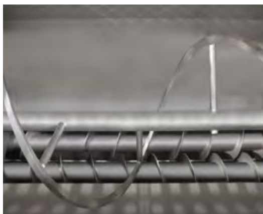
Top view and inside look of the TSF. Both the twin screws and the feeding wing is shown.
