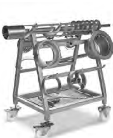
Accessory/cleaning trolley with space for all loose grinder parts.
