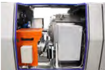
Built-in oil cooler.
