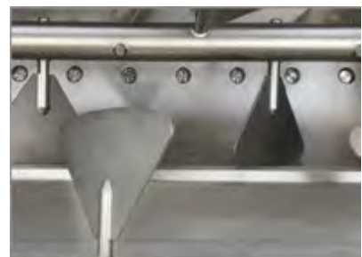
Paddle mixing wings, special application.
