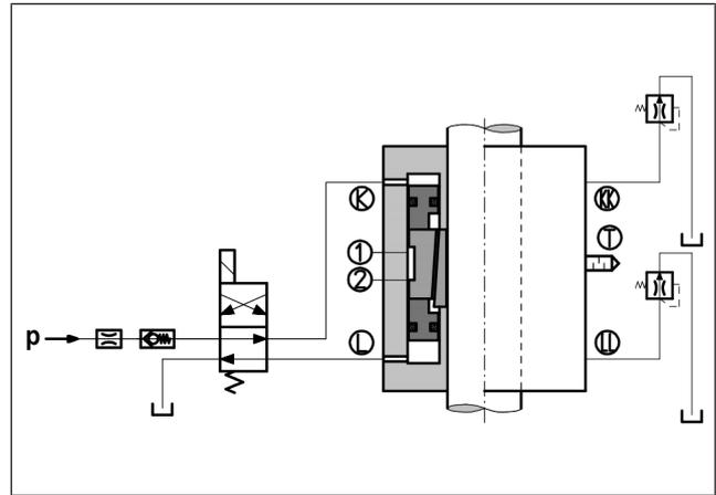
Fig. 3: Example of actuation of Locking Unit
