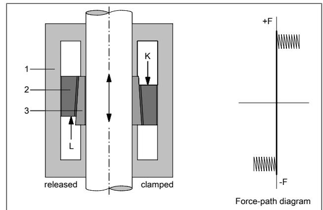
Fig. 1: Functional basics of a Locking Unit
