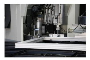
11 pieces of profile cleaning blade and two independed cleaning unit, cleaning bottom, top, interior and external surfaces of the profile.
