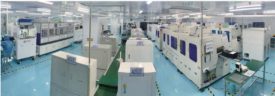
Full-auto COG Bonding Line Full-auto OCA Bonding Line
