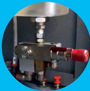
LUBRICANT TANK Integrated lubrication system of the vacuum valves.
