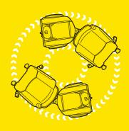
Superb manoeuvrability Our innovative articulated steering makes possible the almost impossible, thus permitting maximum flexibility. As a result, the rear vehicle always runs exactly in the track of the front vehicle. Thanks to this extreme manoeuvrability and the 100% directional stability, it is easy to drive around every obstacle and every kerb. Guaranteed without hitting anything.
