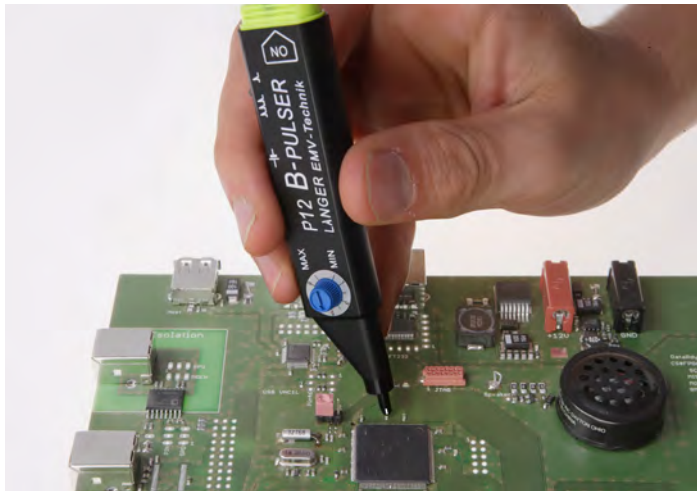
Figure 3 Magnetic field coupling into the VDD systems of an IC
